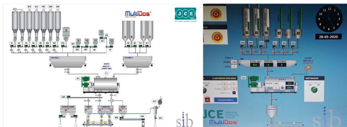
Figure 1: Production Process of the Mortars and Hardeners (PP2) (line 1 left, line 2 right).
